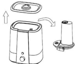
Notes: In the case of hard water (the tap water contains too much calcium and magnesium), limescale deposits can occur in the humidifier and especially in the area of the evaporator and the water vapour unit and these can lead to impairment of the functioning. We therefore recommend that you
